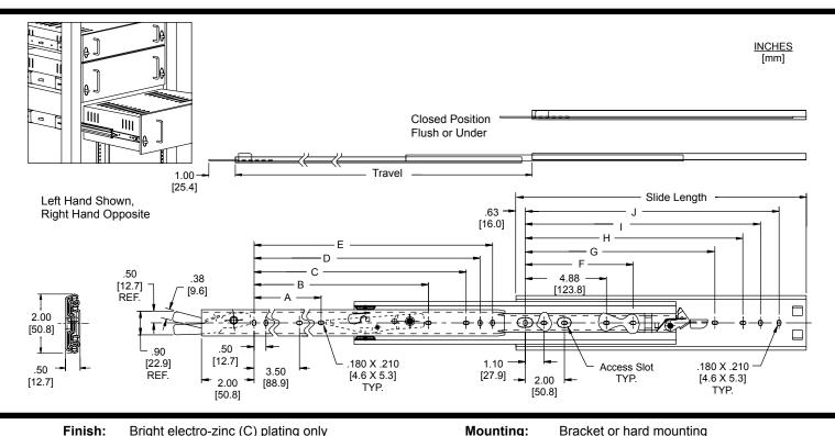
Bright electro-zinc (C) plating only Mounting: Bracket or hard mounting
